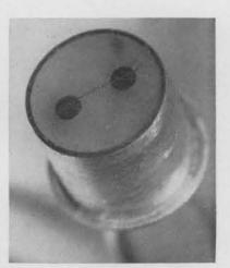
SAMPLE of ultrasonic welding above shows tiny .0008 inch nickel alloy bridgewire joined to Kovar posts .040 in diameter.
